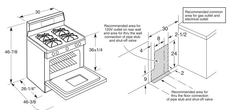
Factory set for Natural gas. A set of LP orifices is included with each range for LP conversion.
